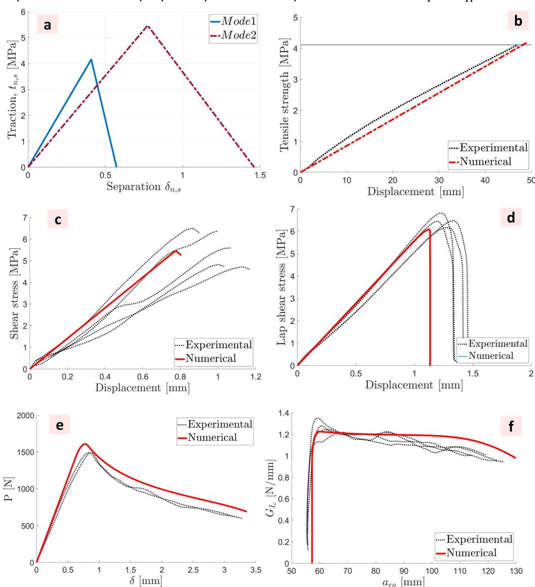
Figure 4 – Experimental versus numerical output data for the tested models: a) triangular shape cohesive law applied; b) tensile test; c) shear test; d) Aluminium SLJ 25 [mm] overlap; e) P- $\delta$  curve for DCB in mode I test; f) R-curve following CBBM
