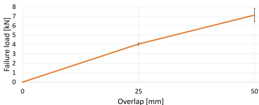
Figure 3 – Failure load vs overlap length for the aluminium SLJs
